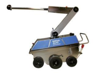
Automatic, self propelled high pressure cleaning robot for stables
