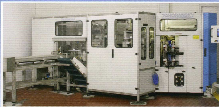
Bürstenstanzmaschine / brush filling machine / machine à estamper
