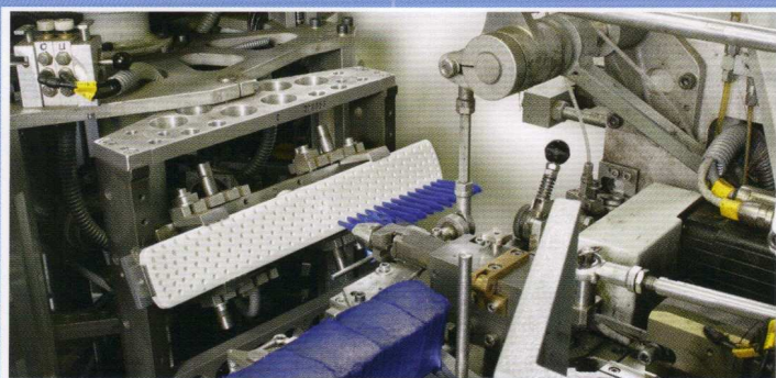
Bürstenstanzmaschine / brush filling machine / machine à estamper
