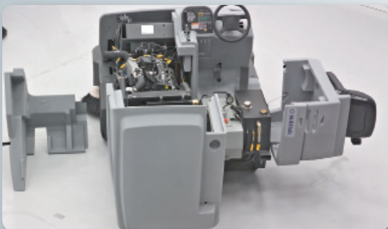
Exceptionally easy serviceability is achieved with Nilfisk's NoTools™ system. The 5-sided access to engine and hydraulic components saves time and keep down the service cost.
