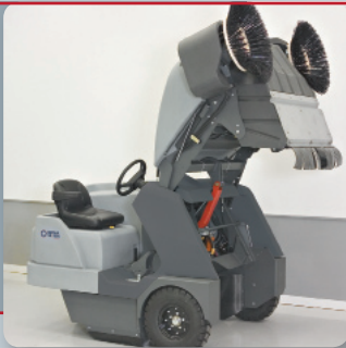
The SR 1900 incorporates superb high-dump capability up to 152 cm from ground level.
